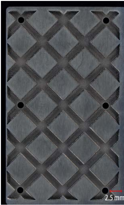
Fig. 4 Combined processing using ultra-short-pulse (trenching) and water-jet guided technology (drilling) from SiC
